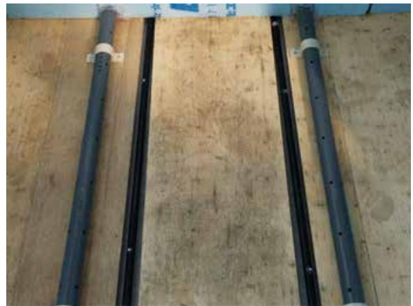
写真-7 テスト槽 (H×W×L = 1,400×1,200×1,000mm)
