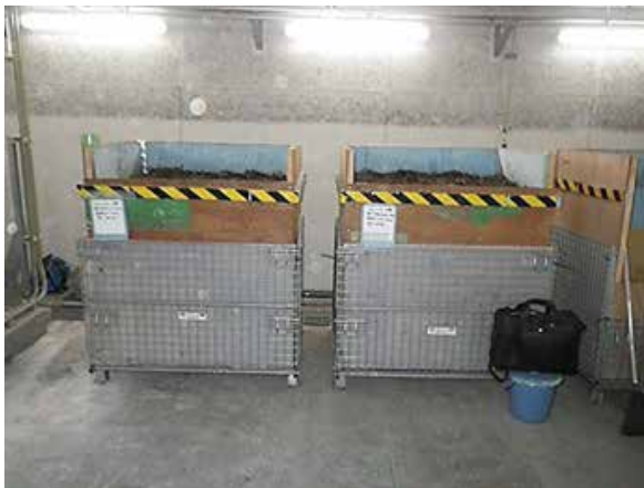
写真-7 テスト槽 (H×W×L = 1,400×1,200×1,000mm)
